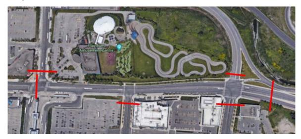
The work is scheduled to commence on July 9, 2018 and will take approximately 15 weeks to complete. This work will involve open excavation within the municipal right of way to install concrete encased ductbank, cable chambers and transformer foundations.
