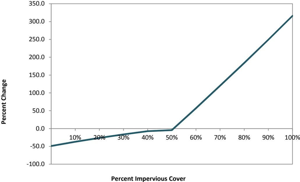
Figure 24: Projected percent change in total flow with changes in percent impervious cover in the Spring Creek subwatershed (based on the 2008 precipitation period).
