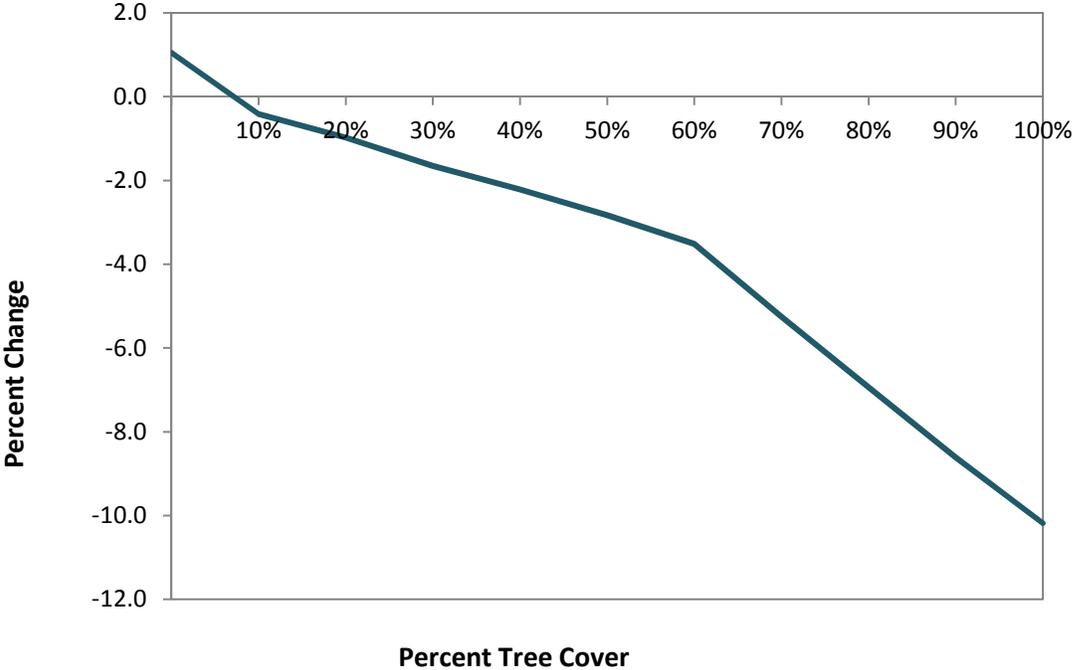
Figure 23: Projected percent change in total flow with changes in percent tree cover in the Spring Creek subwatershed (based on 2008 precipitation period).
